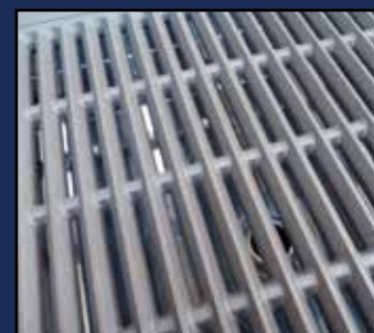
Rack plate, with cast iron bars
